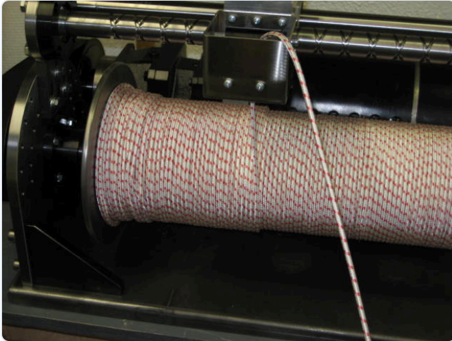
Purpose-built LINEX winch drum and line-management assembly. The large spool carries up to 3,000 ft of 5/32 in aramid-fiber line.
